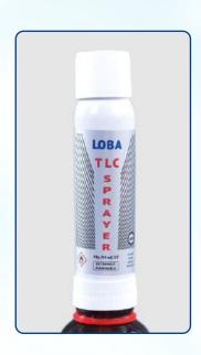
The TLC Sprayer is based on simple technology where the aerosol compartment is situated above the reservoir. A small press of the lever lightly pressurises the lower glass reservoir releasing a fine mist of spray. Gas canister serves as handle; cap fits standard 38-400 thread reagent bottles.
