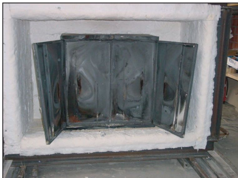
▲ 793 model after fire resistance of 105 minutes. The internal part of the cabinet remained completely fireproof during the whole test
