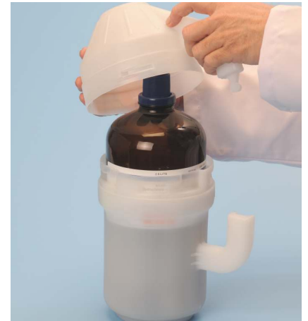
Step 3. Lower the Safe-Handle top over the neck of the bottle. Line up the indicator arrows to ensure proper assembly.
