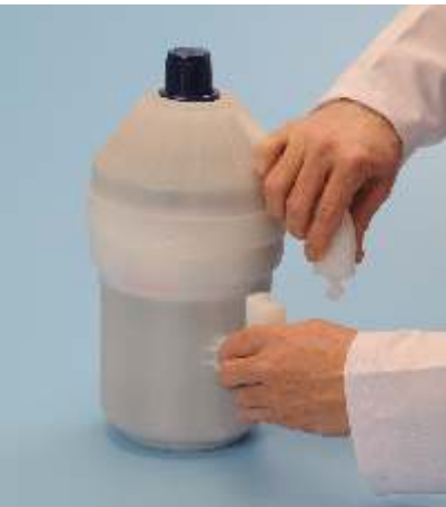
Step 4. While holding the bottom handle with one hand, turn the top handle with the other hand in a clockwise direction until the lugs click into place.
